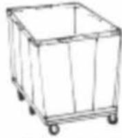
Dandux Workhorse Trucks (400-580 Series). Workhorse, the name says it all !!! The Dandux Workhorse Truck is the commercial version of the Dandux Postal Spec Truck. Built for use in extremely heavy workload and abusive environments. Constructed with extra heavy white canvas laced to an electro welded spring steel frame. Six high quality 4" casters with thread guards are mounted to kiln dried hardwood runners and caster boards.
